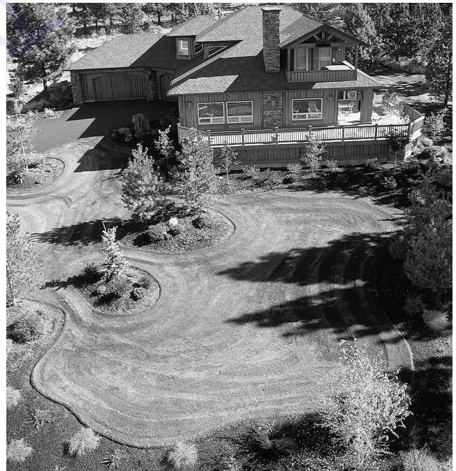
FIGURE A.17.1.9.2(b) Small Planting Islands Within an Expanse of Maintained Lawn. (Courtesy of Firewise Communities Program. Photo by D. Frazier.) [1144:Figure A.4.2.5.2(b)]
