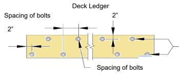
Example of correct placement of fasteners in deck ledgers (rim joists). Bolts must be placed in the deck ledgers as shown. Spacing of fasteners per table R507.2.
